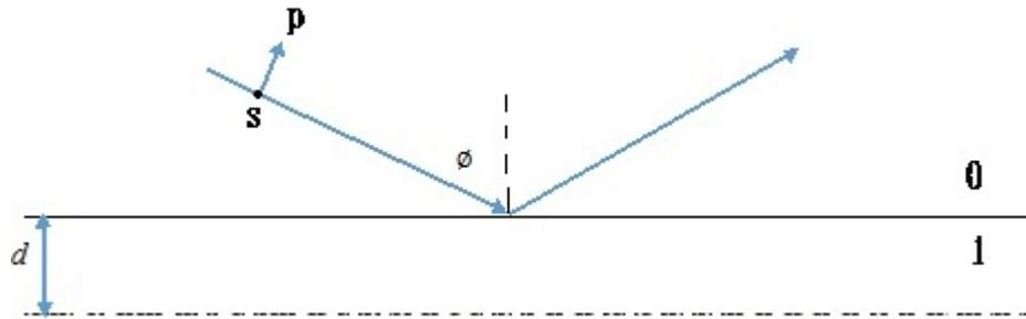
FIG. 1. Reflection of  $p$ - and  $s$ -polarized light at the interface between two transparent media 0 and 1. Reflectance enhancement due to the coherent interference of light within a truncated slab of thickness  $d$  (and exit medium 0) is the subject of this paper. In this figure, the  $s$  polarization is normal to the page; i.e., the plane of incidence.
