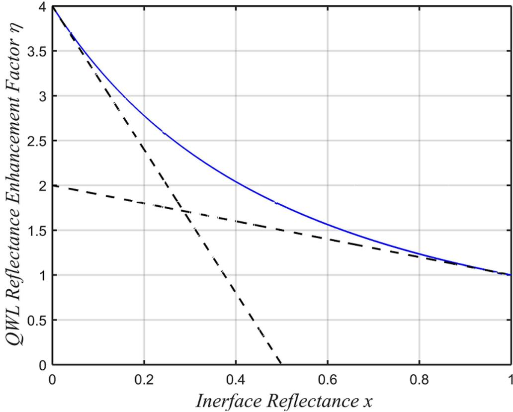
FIG. 2. Reflectance enhancement factor  $\eta$  [Eq. (8)] due to coherent interference of light in a QWL is plotted as a function of the intensity reflectance of the ambient-layer interface  $x = r_{01v}^2$ .
