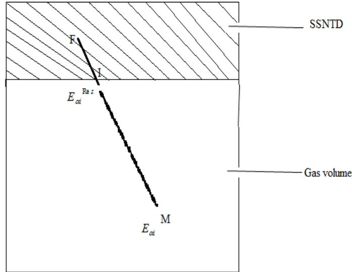
FIG. 6. Diagram illustrating primary trajectory of an  $\alpha$ -particle inside the gas volume (MI = X) and SSNTD (IF = RD).  $E_{\alpha i}$  is the initial energy of the  $\alpha$ -particle and  $E_{\alpha i}^{\text{Res}}$  is its residual energy on reaching point I.
