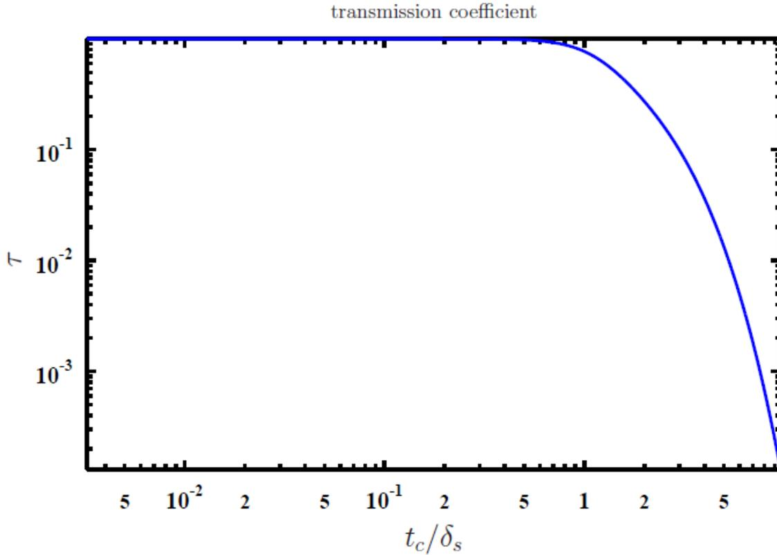
FIG. 3. Transmission coefficient  $\tau$  (log scale) as a function of the normalized conducting wall thickness  $t_c/\delta_s$ . The parameters used are: circumference  $L = 125$  m, pipe radius  $b = 10$  cm, beam radius  $a = 5$  cm, dielectric thickness  $t_d = 3 \mu\text{m}$  and  $\kappa_d = 6$ , injection energy  $\gamma_0 = 1.02$ , harmonic number  $n = 5$  and reference frequency  $\omega_0 = 2.41 \times 10^6$  rad/s.
