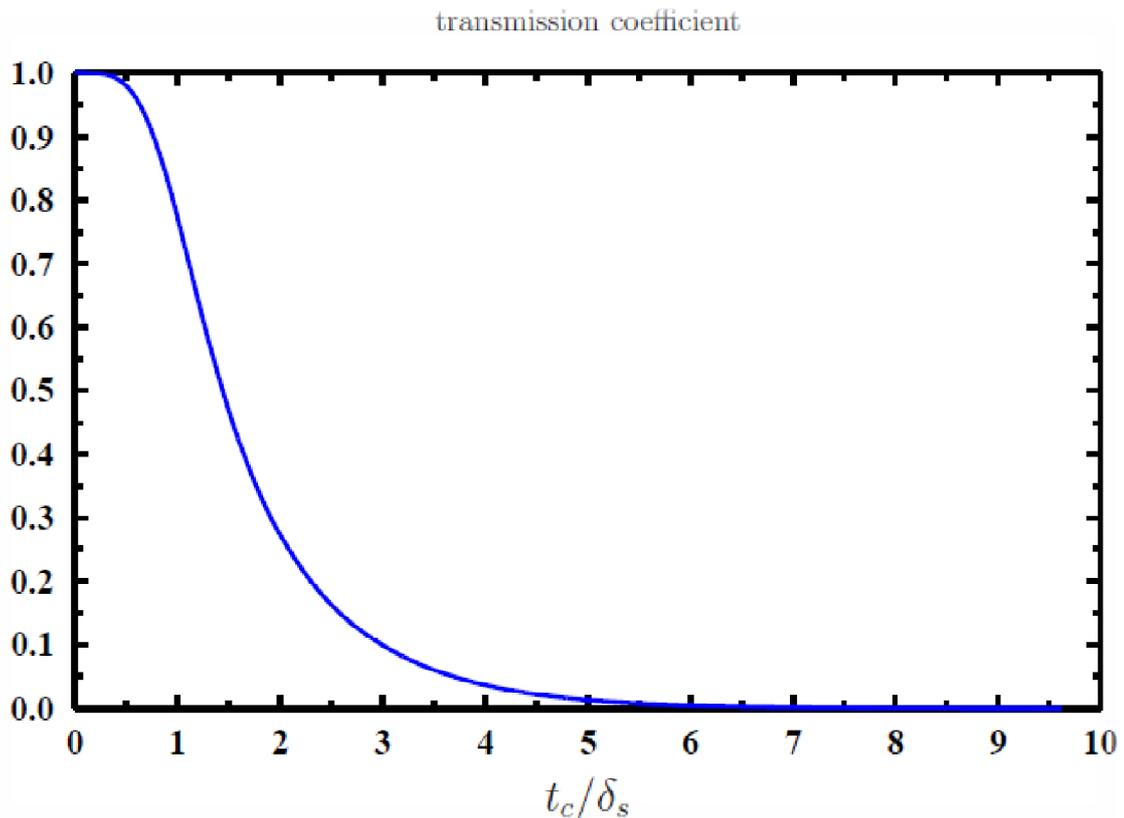
FIG. 2. Transmission coefficient  $\tau$  as a function of the conducting wall thickness  $t_c/\delta_s$ . The parameters used are: circumference  $L = 125$  m, pipe radius  $b = 10$  cm, beam radius  $a = 5$  cm, dielectric thickness  $t_d = 3$   $\mu\text{m}$  and  $\kappa_d = 6$ , injection energy  $\gamma_0 = 1.02$ , harmonic number  $n = 5$  and reference frequency  $\omega_0 = 2.41 \times 10^6$  rad/s.
