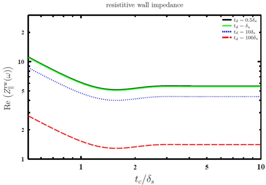
FIG. 4. Real part of the resistive-wall impedance in  $\Omega$  as a function of the conducting wall thickness  $t_c/\delta_s$ . The parameters used are: circumference  $L = 125$  m, pipe radius  $b = 10$  cm, beam radius  $a = 5$  cm, dielectric constant  $\kappa = 6$ , injection energy  $\gamma_0 = 1.02$ , harmonic number  $n = 5$  and reference frequency  $\omega_0 = 2.41 \times 10^6$  rad/s.
