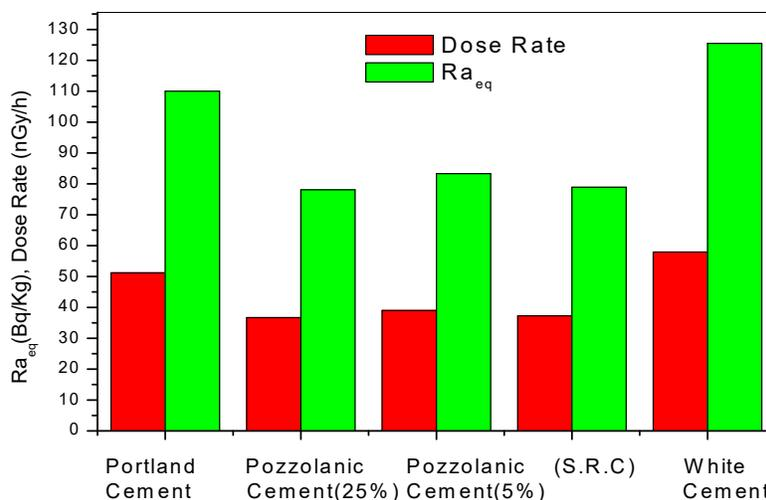
FIG. 2. Comparison between the average values of radium equivalent,  $Ra_{eq}$ , and dose rate in different kinds of cement in Jordan.
