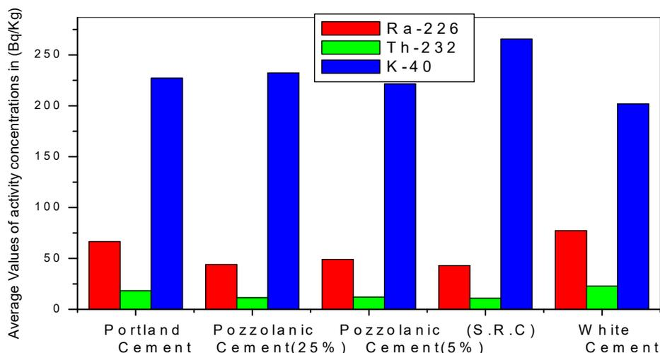
FIG. 1. Different kinds of cements vs. activity concentrations (Bq.kg<sup>-1</sup>).
