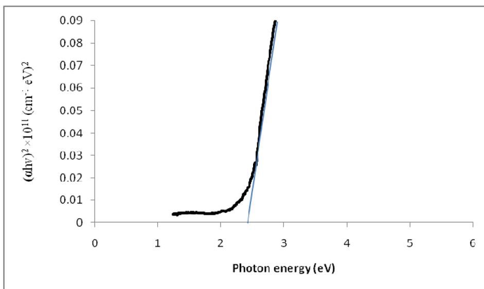
FIG. 6. Band gap of 100 nm CdS film.
