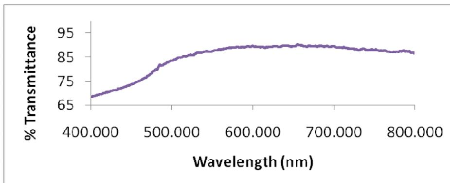
FIG. 4. % transmittance characteristics of 100 nm CdS film.
