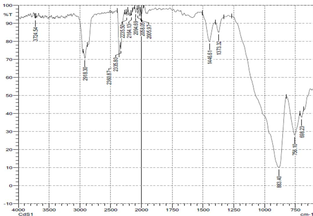
FIG. 7. FTIR for the 100 nm CdS film.
