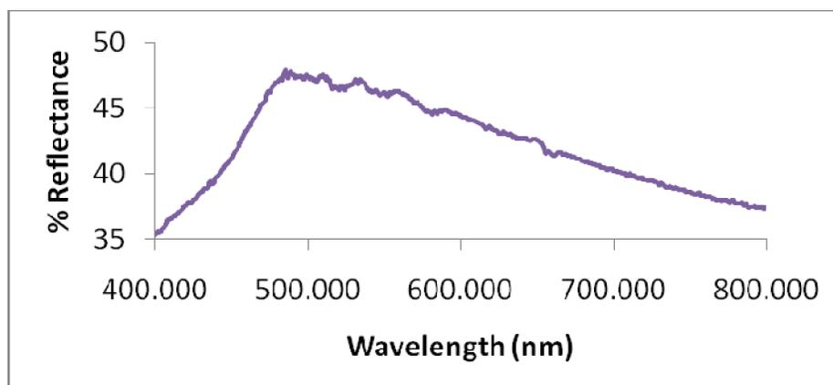
FIG. 3. % reflectance characteristics of 100 nm CdS film.
