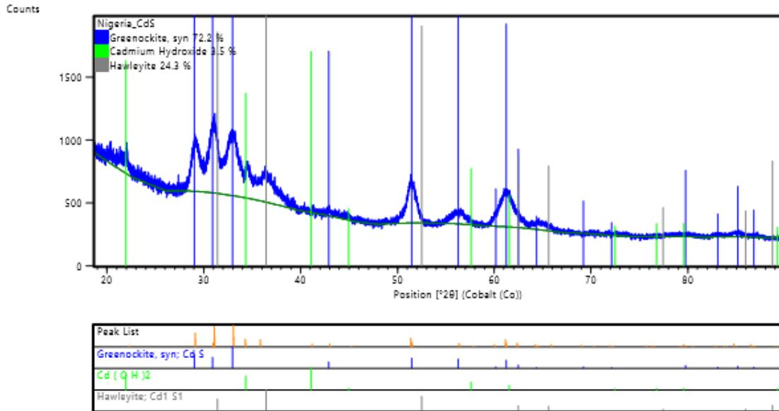
FIG. 1. XRD analysis of the synthesized CdS nano-particles.
