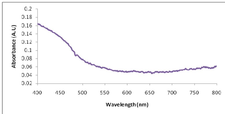
FIG. 5. % absorbance characteristics of 100 nm CdS film.
