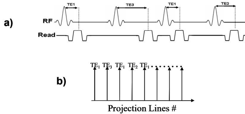
FIG. 1. a. The modified TrueFISP sequence. b. The acquired projections with different echo times are spaced by an angle increment of 111.246°.
