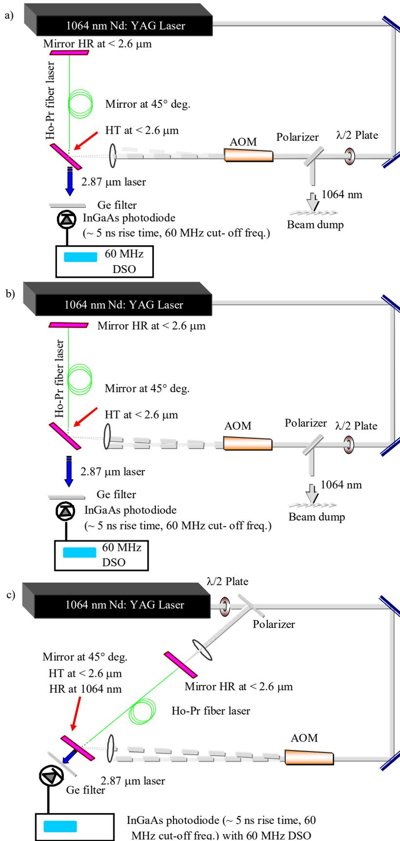
FIG. 1. Experimental setups for pulse pumping a single-clad Ho<sup>3+</sup>, Pr<sup>3+</sup> co-doped ZBLAN fiber laser. a) Zero order AOM operation, b) first order AOM operation, c) first order AOM operation with simultaneous CW pumping of the second fiber facet.
