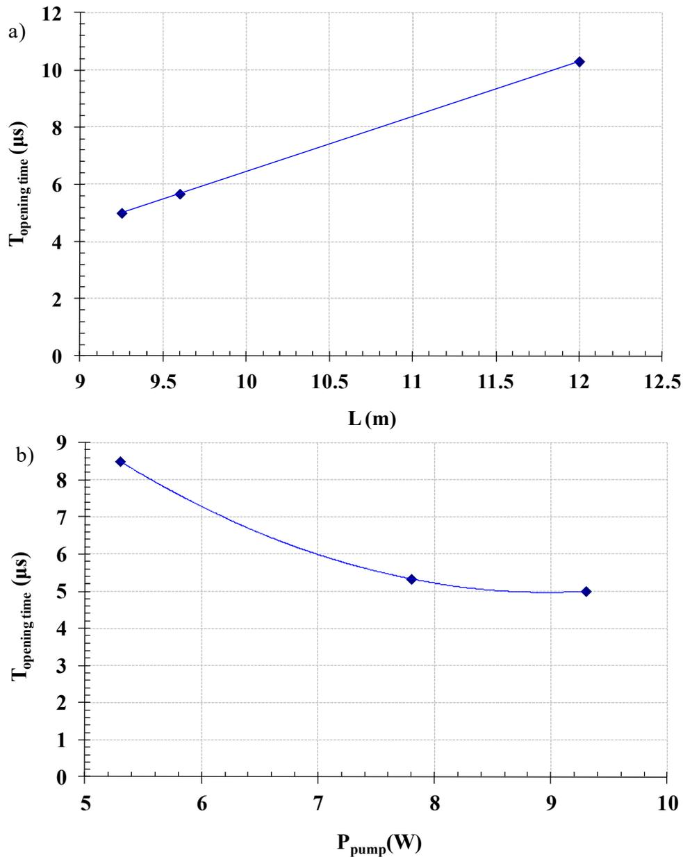
FIG. 2. Opening time of zero order AOM operation required to produce a single pulse at 50 kHz modulation frequency as function of a) fiber length, b) pump power.
