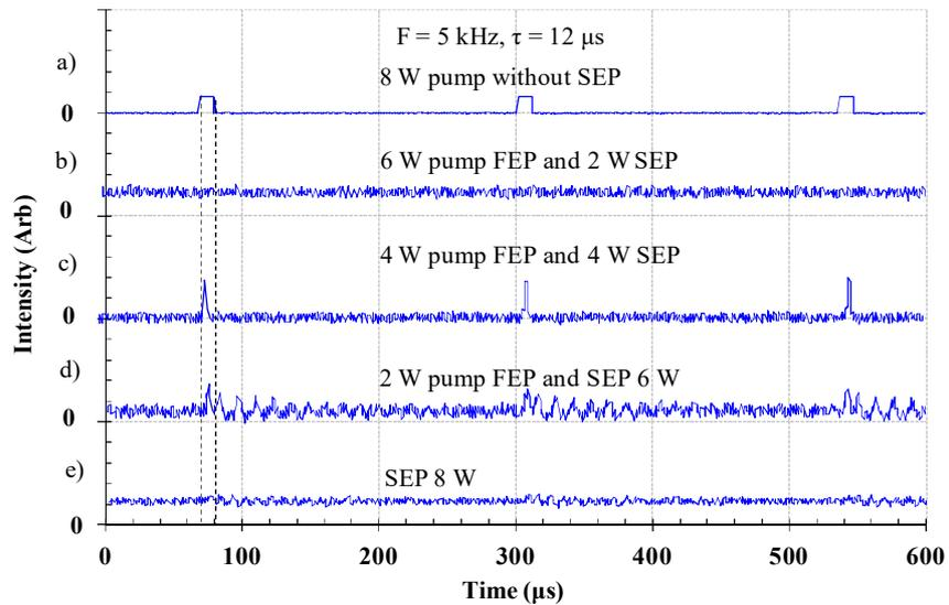
FIG. 6. Temporal profiles of the output of the laser for changes in the degree of double end pumping, first order AOM operation for fiber length of 1.5 m. a) CW output, when small opening time applied with single end pumping (SEP), b) train of pulses when less than 2 W second facet pumping (SFP) applied, with 6 W first end pump (FEP) c) train of relaxation oscillations for 4W SFP, d) quasi-CW and CW output with less than 6W SFP pump.
