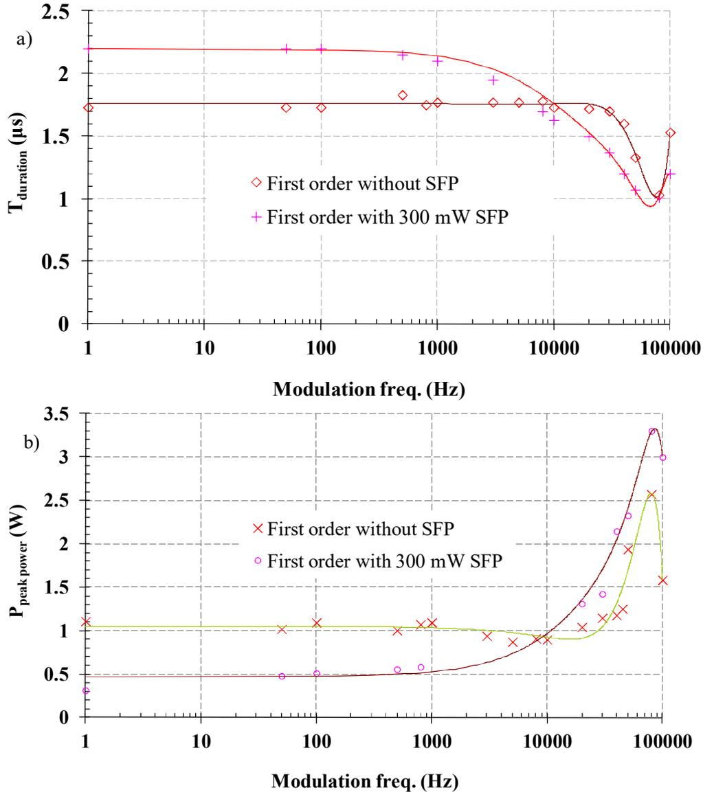
FIG. 7. The comparison between a) pulse durations and b) peak powers as a function of modulation frequency for first order AOM operation with 300 mW SFP and without SFP respectively.
