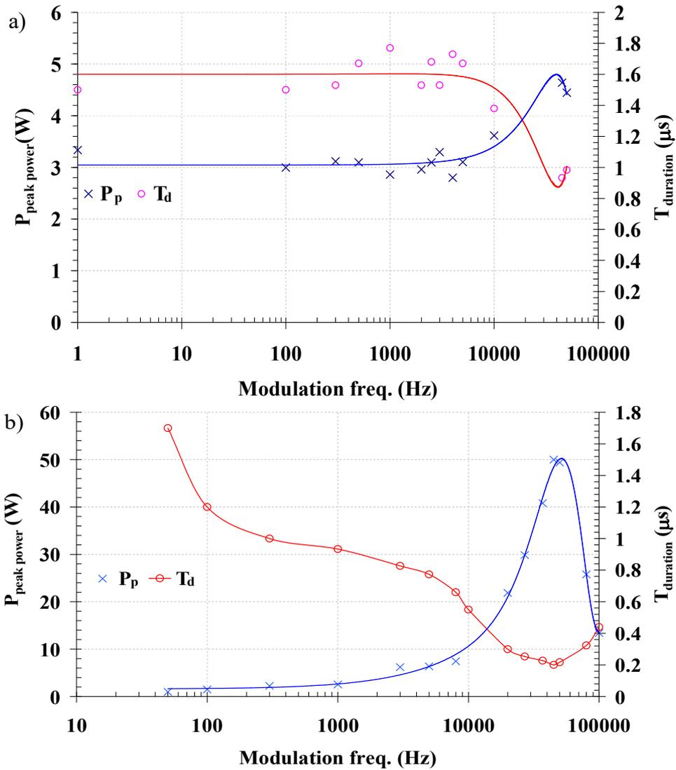
FIG. 3. Peak power and pulse duration as a function of modulation frequency for zero order AOM operation and for a) 12 m fiber length and 9.3 W pump power, b) 9.25 m fiber length and pump power of 9.3 W.
