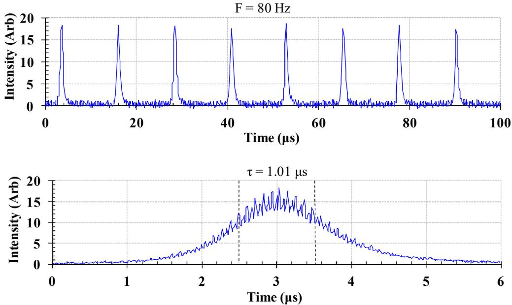
FIG. 8. Temporal profiles for first order AOM operation: a pulse train with modulation frequency of 80 kHz and a single pulse with duration of 1.01  $\mu\text{s}$ .
