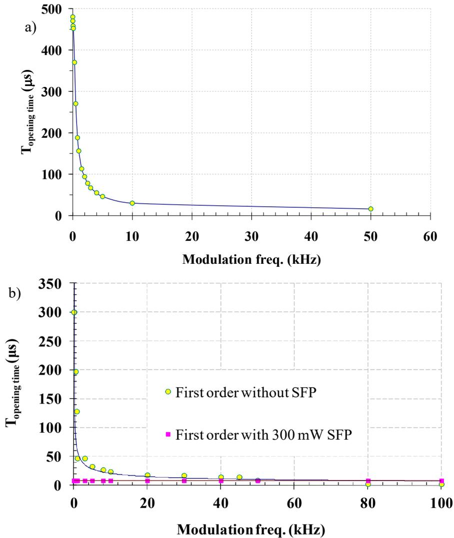
FIG. 5. Opening time as a function of frequency modulation for first order AOM operation, (a) 13.25 m fiber length, b) 9.25 m fiber length, without second facet pumping (SFP) and with 300 mW SFP.
