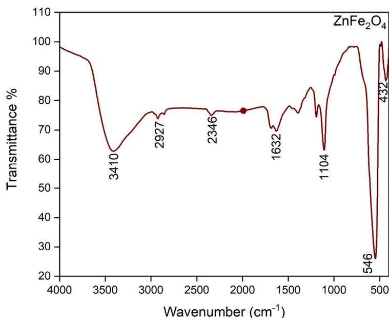
Fig. 2. FTIR pattern of ZnFe<sub>2</sub>O<sub>4</sub>.
