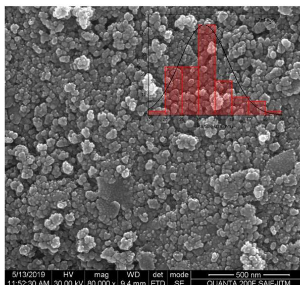
Fig. 4. Particle size distribution of  $\text{ZnFe}_2\text{O}_4$ .
