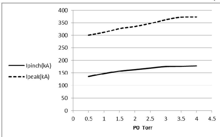
FIG. 6. Effect on total current ( $I_{peak}$ ) and pinch current ( $I_{pinch}$ ) as  $P_0$  is increased from 0.5 to 4 Torr.
