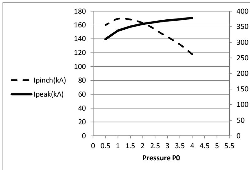
FIG. 3. Variation of  $I_{pinch}$  and  $I_{peak}$  versus pressure.
