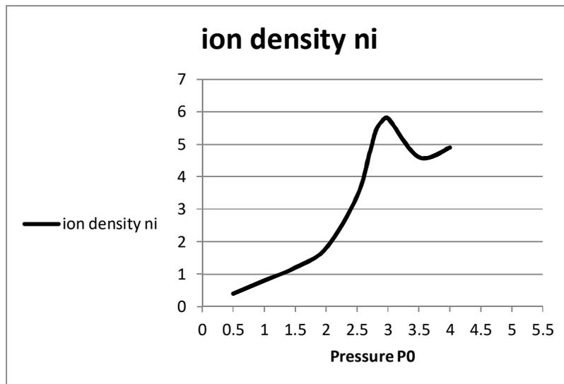
FIG. 4. Variation of ion density versus pressure.
