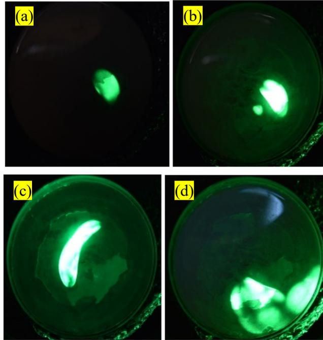
FIG. 6. Images of field-emission currents for the uncoated tungsten tip. The  $I_m(V_m)$  data for each photograph is: (a) (630 V, 1.5 nA), (b) (710 V, 30 nA), (c) (850 V, 240 nA) and (d) (990 V, 750 nA).
