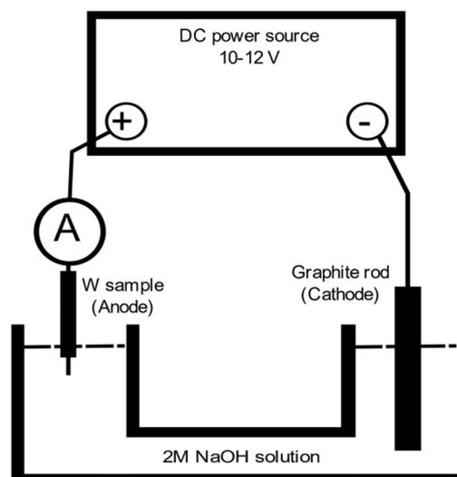
FIG. 2. Schematic diagram for the etching device.
