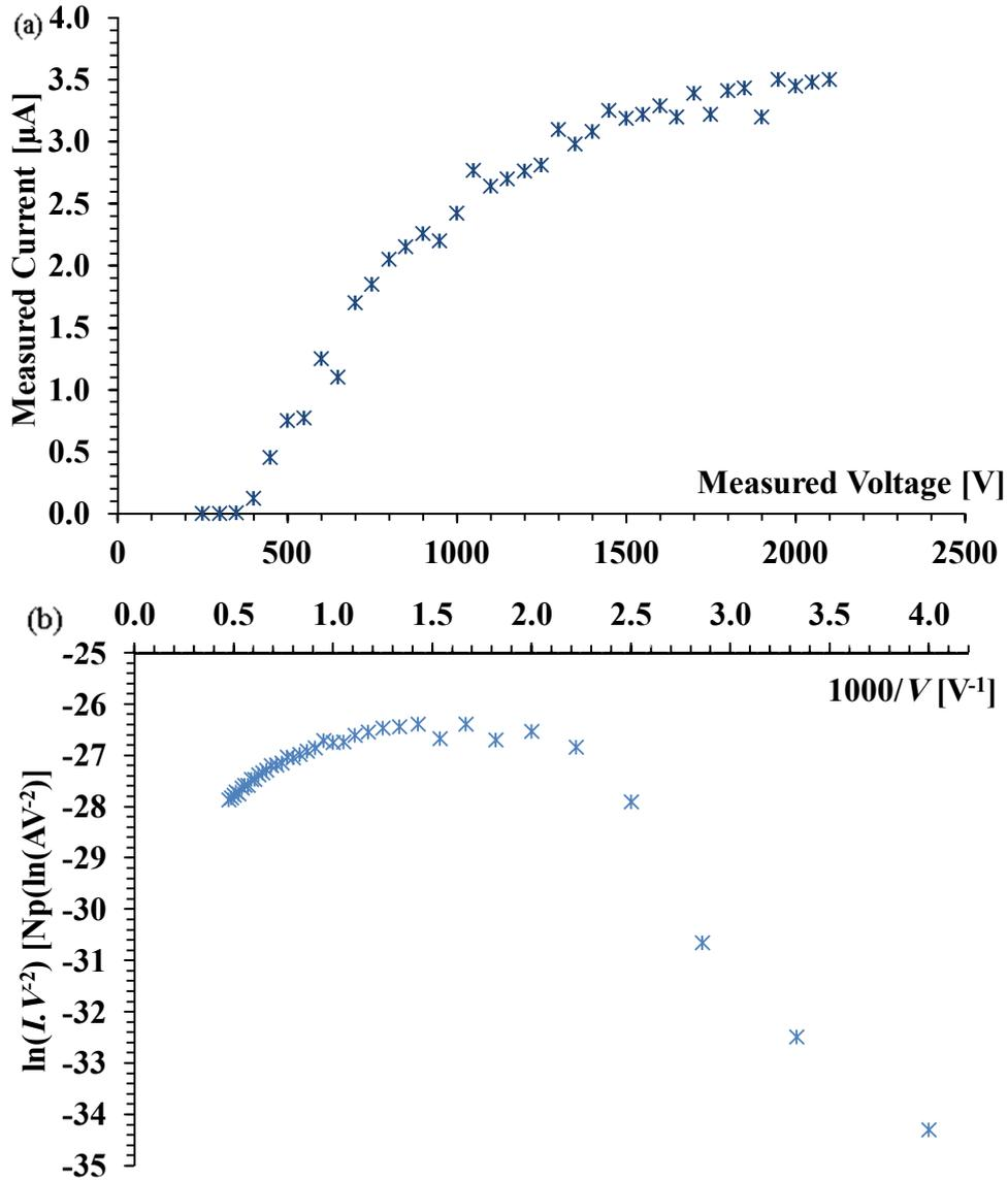
FIG. 7. (a) The current-voltage characteristics for the composite sample during the first voltage-decreasing interval with  $V_{\text{sw}} = 2100 \text{ V}$ ,  $I_{\text{sat}} = 3.5 \mu\text{A}$  and (b) The related Fowler-Nordheim plot.
