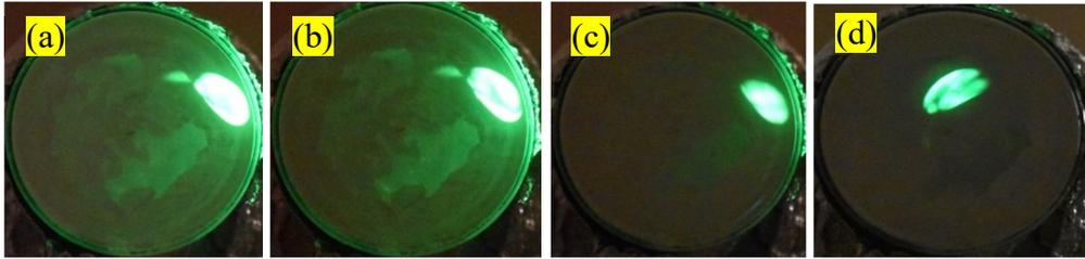
FIG. 10. Field-emission microscope images obtained for the composite sample during the first decrease interval. The current-voltage data for each image is: (a) (980 V, 2.3  $\mu$ A), (b) (880 V, 2.22  $\mu$ A), (c) (790 V, 1.87  $\mu$ A) and (d) (700 V, 1.63  $\mu$ A).
