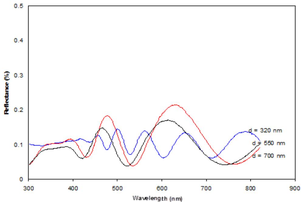
FIG. 3. The reflectance (R) curve as a function of wavelength of three  $V_2O_5$  films ( $d = 320, 550$  and  $700$  nm)
