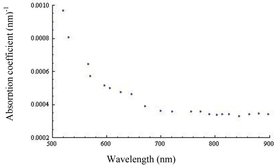
FIG. 10. Absorption coefficient of the as deposited  $V_2O_5$  (700 nm) thin film against wavelength
