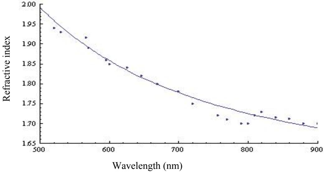
FIG. 8. Refractive index of  $V_2O_5$  (700 nm) film versus wavelength (dot points for measured and line for fitting)
