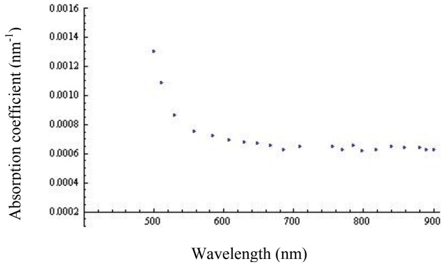
FIG. 6. Absorption coefficient of an as deposited  $V_2O_5$  (320 nm) thin film against wavelength
