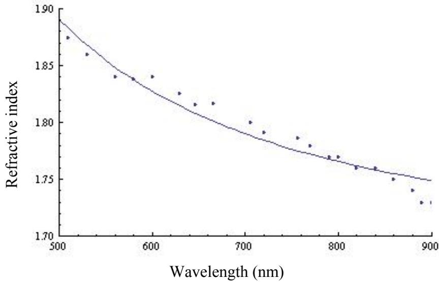
FIG. 4. Refractive index of  $V_2O_5$  film (320 nm) versus wavelength. The points represent the calculated values and the full curve is the fitting curve according to Eq. 4
