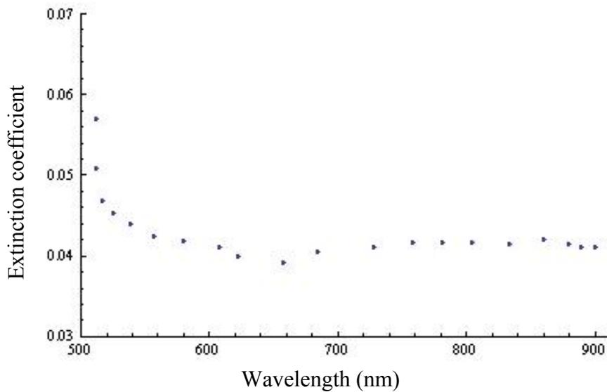
FIG. 5. Extinction coefficient of an as deposited  $V_2O_5$  (320 nm) thin film against wavelength
