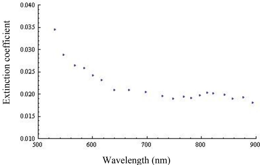
FIG. 9. Extinction coefficient of the as deposited  $V_2O_5$  (700 nm) thin film against wavelength
