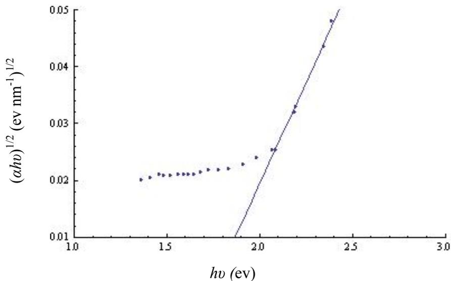
FIG. 11.  $(\alpha h\nu)^{1/2}$  versus  $(h\nu)$  plot for 700 nm  $V_2O_5$  thin film
