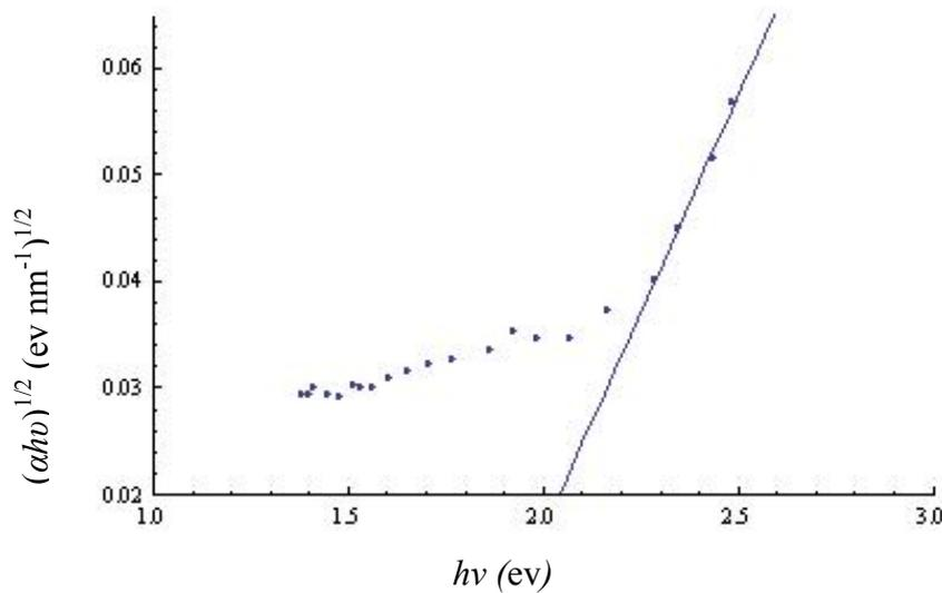
FIG. 7.  $(\alpha hv)^{1/2}$  versus  $(hv)$  plot for 320 nm  $V_2O_5$  thin film
