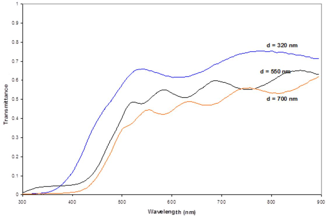
FIG. 2. The transmittance (T) curve as a function of wavelength of three  $V_2O_5$  films ( $d = 320, 550$  and  $700$  nm)
