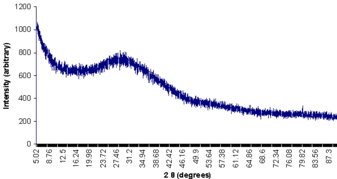
FIG. 1. X-ray diffraction pattern of an as deposited  $V_2O_5$  thin film on a glass substrate
